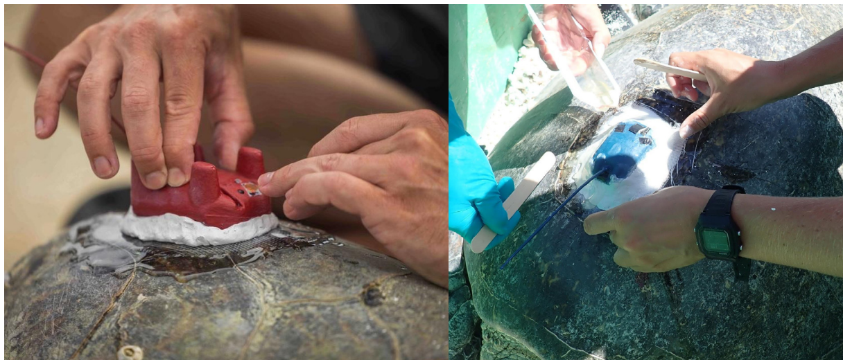
Figure 33. 33a.) Attaching a satellite transmitter using a marine putty base. 33b.) Adding marine putty to the area surrounding the transmitter to create a more hydrodynamic profile. Photos courtesy of NMFS PIFSC, NMFS Permit 21260.
