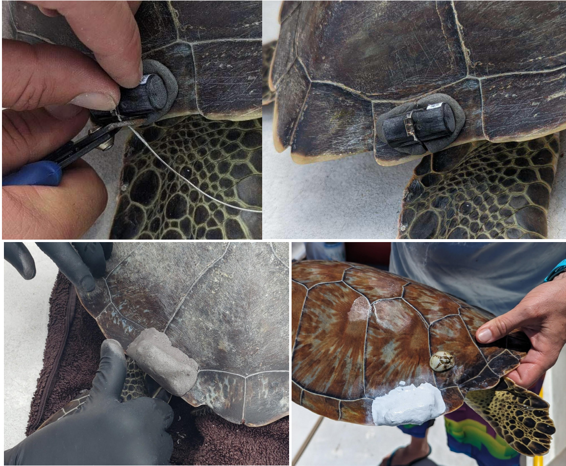
Figure 36. Attaching an acoustic transmitter to the flattest section of the post-marginal scutes, approximately 10–15 millimeters from the edge of the scute. The tag is attached after drilling an 4 to 8-millimeter hole with a sterilized drill bit. 36a.) Initial tag attachment to plumber's putty base. A tie is inserted through the drilled hole and the extra tie length is then removed. 36b.) Tag after extra tie length is removed. 36c.) Building up putty over the tag to create a more hydrodynamic profile. 36d.) Anti-fouling paint can be applied to the tag for extra protection. Photos courtesy of IRG, NMFS Permit 25696/21169, FWC MTP 125/204.
