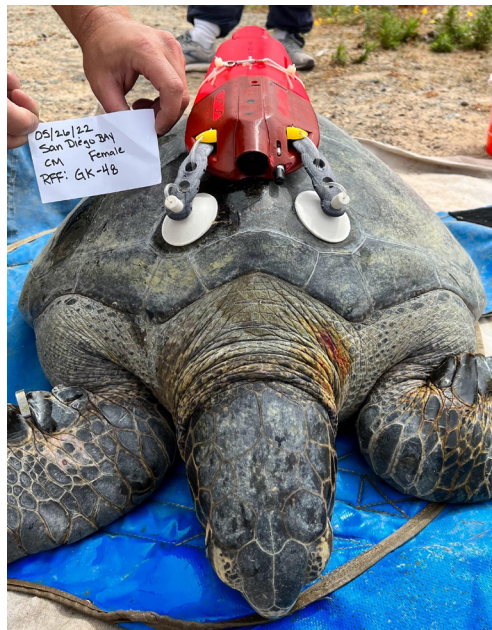
Figure 31. AVED tag attached via suction cup to a hard-shelled turtle. Photo courtesy of NMFS SWFSC, NMFS Permit 18238.
