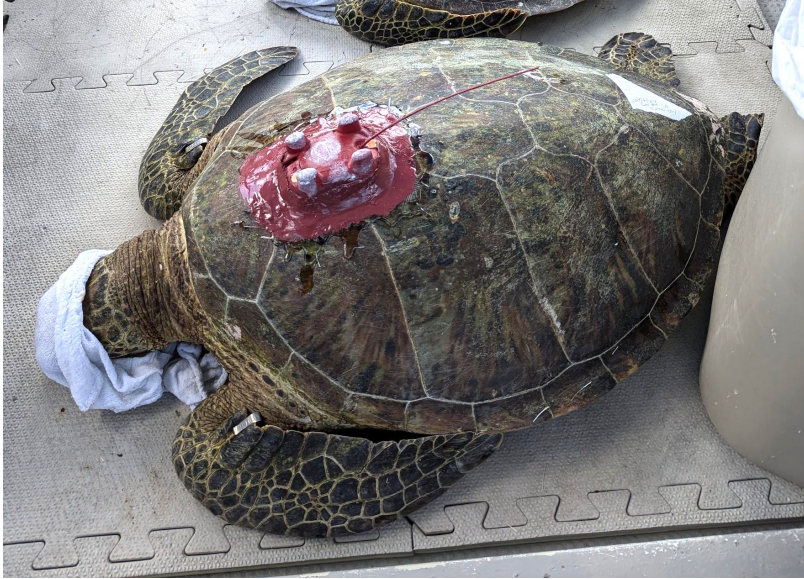
Figure 35. Anti-fouling paint applied to a transmitter and attachment materials and not directly to the carapace. Photo courtesy of NMFS PIFSC, NMFS Permit 21260.
