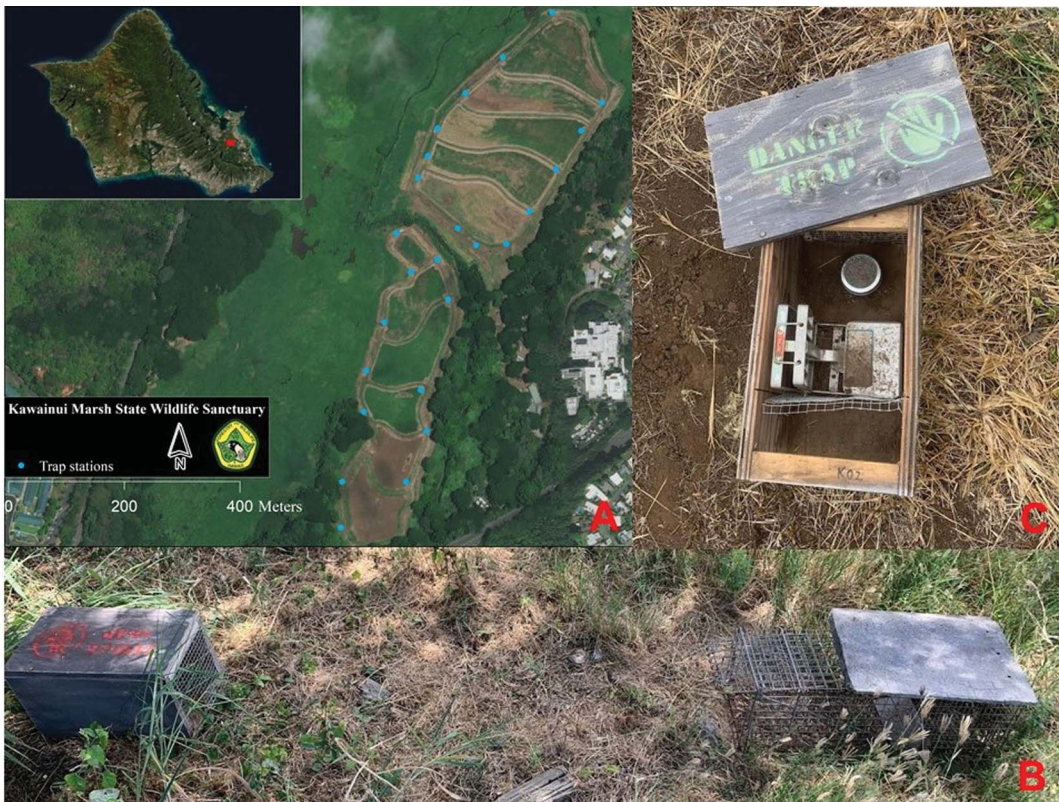
FIGURE 1. (A) Trapping locations of DOC-200 and Tomahawk trap pairs on access roads at the restoration ponds at Kawaiinui Marsh State Wildlife Sanctuary, Kailua, O'ahu, Hawai'i, USA. (B) DOC-200 trap and Tomahawk trap spaced 2 m apart, with entrances facing each other. (C) Inside DOC-200 trap, trap entrance at bottom with 8 \times 8 cm hole, leading into mesh screen with 8 \times 8 cm hole in front of DOC-200, stainless-steel DOC-200 trap triggered when stepped on, followed by bait jar.
