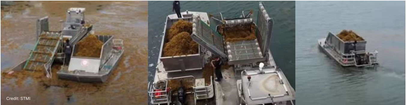
Sargator-2 harvest boat simultaneously collecting and off-loading to coupled transport vessel. Outfitted for two transport vessels and recent tests show a collection capacity of 100 tons per hour
