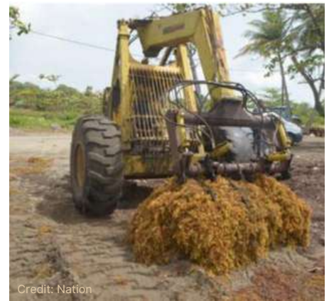
Sugar cane grabs have been used successfully for lifting sargassum
